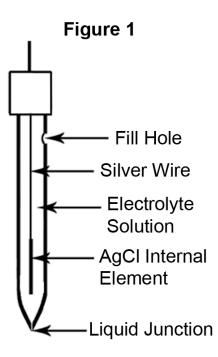
Figure 1 to the left shows the various parts of a typical reference electrode.
